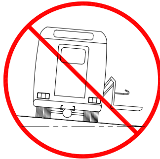
FIGURE 2-1: SLOPED PARKING HAZARD
