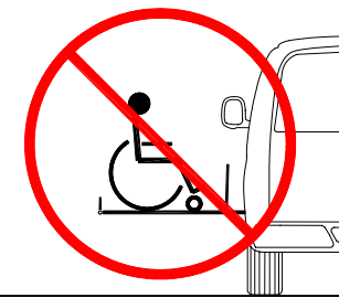
FIGURE 2-2: ALWAYS FACE OUTBOARD WHEN RIDING ON THE LIFT PLATFORM
