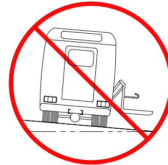
FIGURE 2-1: SLOPED PARKING HAZARD
