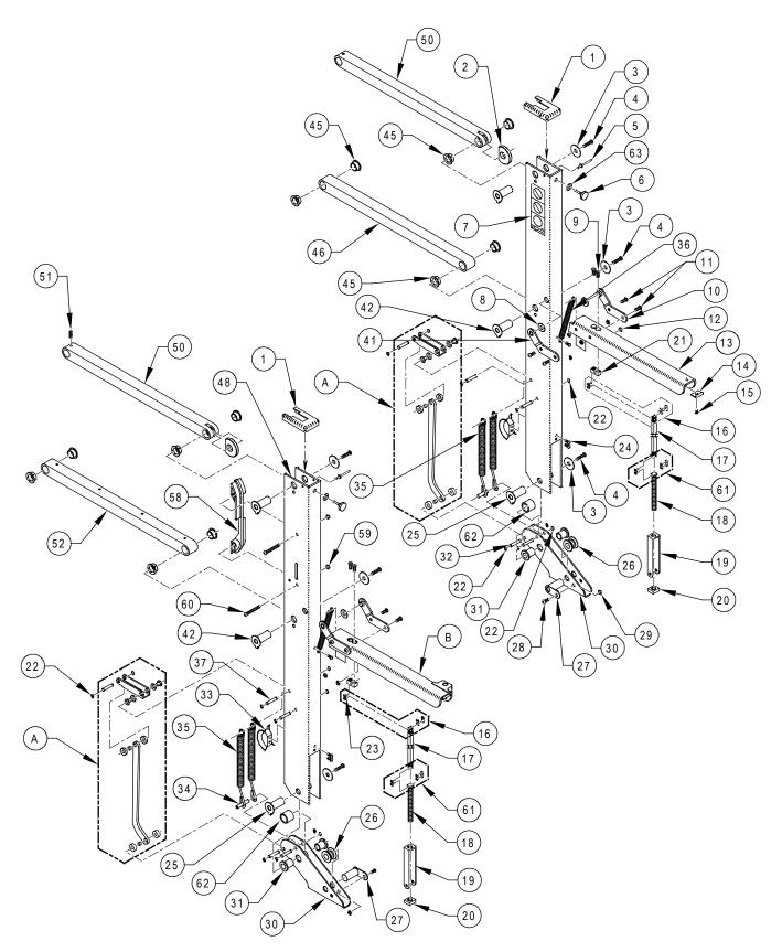
FIGURE 4-4: UNI-LITE PLATFORM POST ASSEMBLY (SHEET 1 OF 2)
