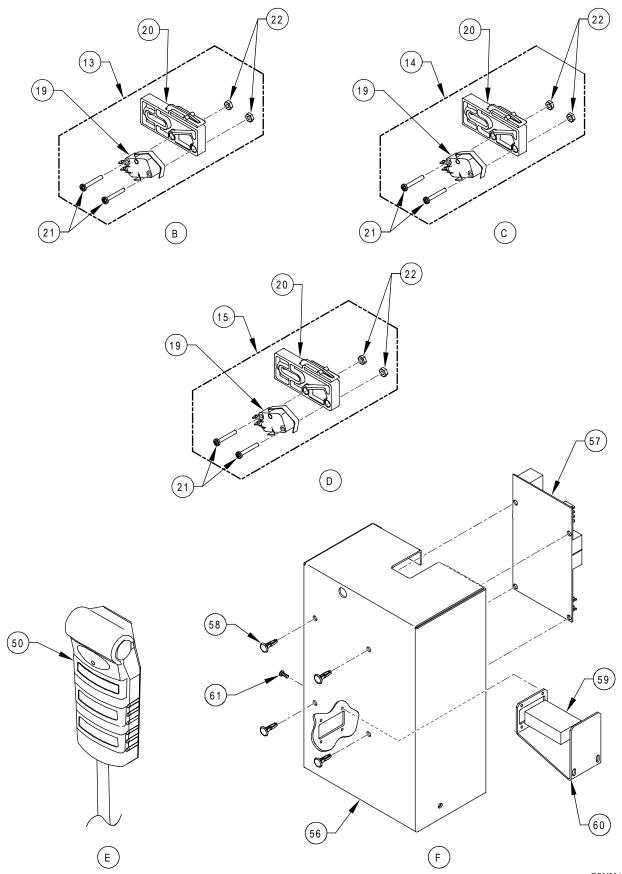
FIGURE 4-3: UNI-LITE ELECTRICAL ASSEMBLY (SHEET 2 OF 2)
