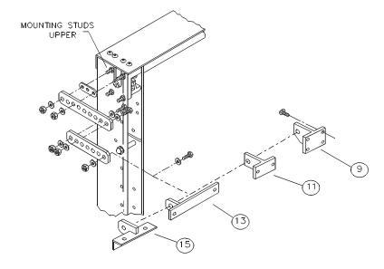
FIGURE 2-14: INTERMEDIATE AND MOUNTING BRACKET INSTALLATION
