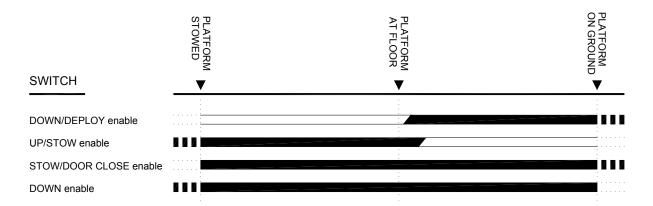
FIGURE 3-3: LIMIT SWITCH ACTUATION DIAGRAM
