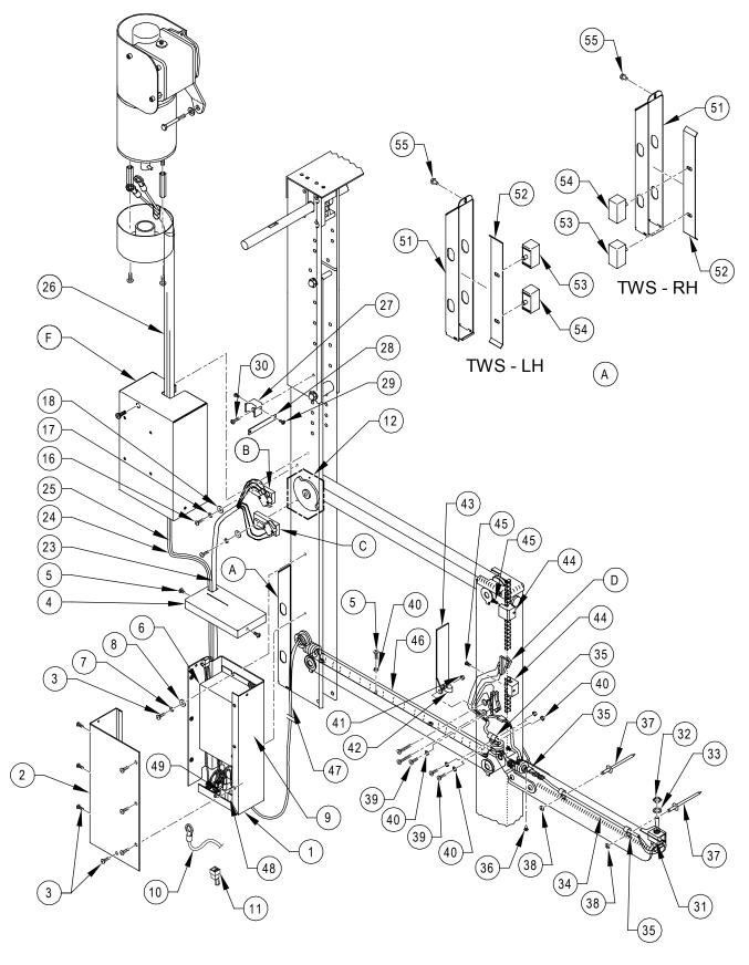
FIGURE 4-3: UNI-LITE ELECTRICAL ASSEMBLY (SHEET 1 OF 2)
