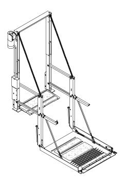
Standard features of the UNI-lite are convenient twin handrails with a control switch, a powerful electric motor and direct gear drive, and a powered roll stop with mechanical latch. The UNI-lite also contains a built-in manual backup system with a manual wrench, and a simple modular electrical system.
