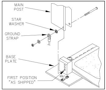
FIGURE 2-10: BASE PLATE MOUNTING
