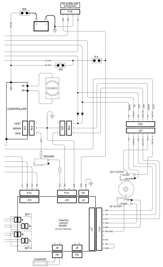
FIGURE 3-6: ELECTRICAL WIRING DIAGRAM - SHEET 2
