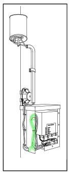
FIGURE 2-2: CONTROLLER WIRE ROUTING DIAGRAM
