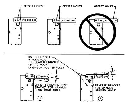
FIGURE 2-13: EXTENSION BRACKET MOUNTING
