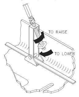
FIGURE 2-17: PLATFORM SUPPORT CHAIN ADJUSTMENT
