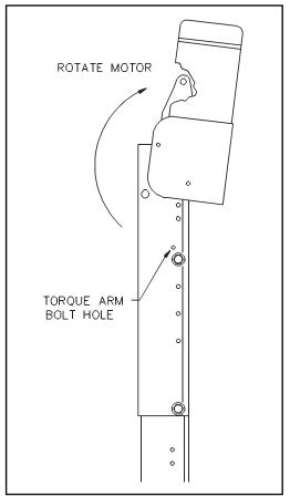
FIGURE 2-7: ROTATE GEAR MOTOR ASSEMBLY
