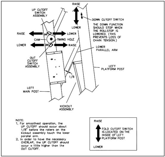
FIGURE 2-18: LIMIT SWITCH ADJUSTMENTS
