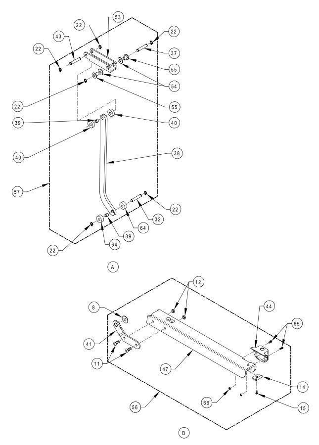
FIGURE 4-4: UNI-LITE PLATFORM POST ASSEMBLY (SHEET 2 OF 2)
