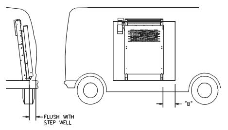
FIGURE 2-11: SIDE DOOR INSTALLATION CLEARANCES
