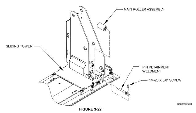
3. Refer to **Figure 3-23**. Pry up on front rail to remove lift weight on roller. Push pin bushings and sleeve out.
