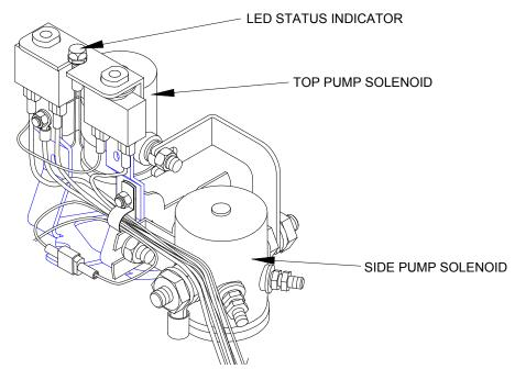
FIGURE 3-2: STATUS INDICATOR FOR PUMP SOLENOIDS
