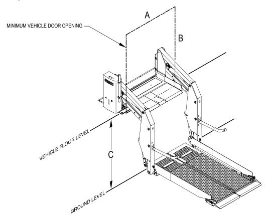
FIGURE 2-1: MINIMUM DOOR SIZE REQUIREMENTS
