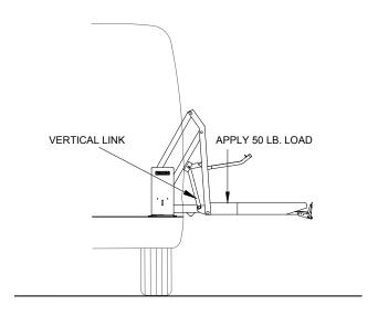
FIGURE 2-15: PRESSURE SWITCH TEST AT FLOOR LEVEL
