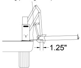
FIGURE 2-13: ADJUSTMENT OF BRIDGEPLATE
