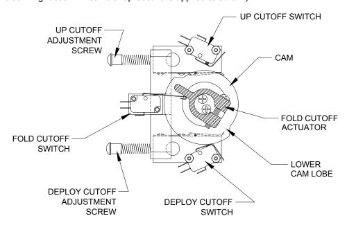
FIGURE 2-9: LIMIT SWITCH ADJUSTMENT DIAGRAM
