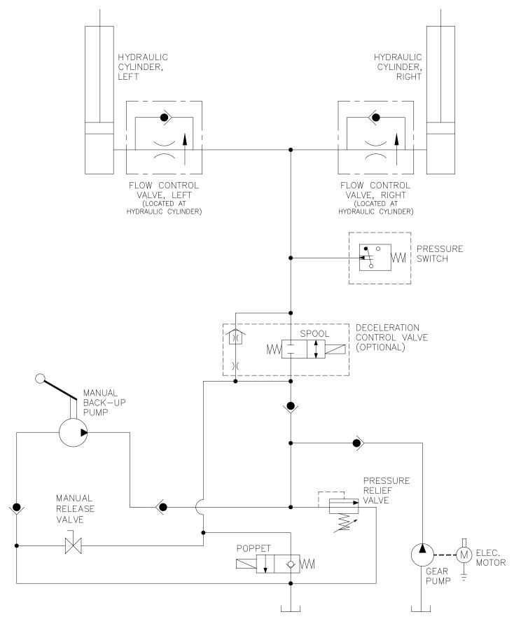
FIGURE 3-43: SLIDE-AWAY HYDRAULIC CIRCUIT DIAGRAM
