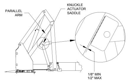
Figure 2-10: knuckle actuator saddle clearance
