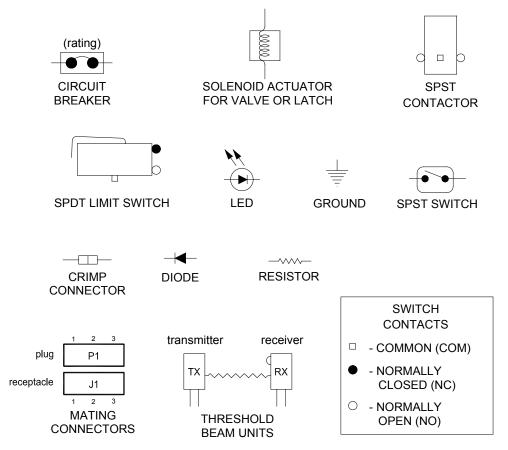
FIGURE 3-45 ELECTRICAL WIRING DIAGRAM SYMBOLS
