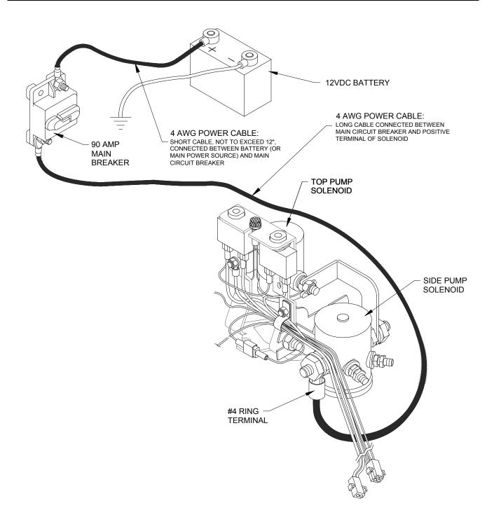
FIGURE 2-4: ELECTRICAL INSTALLATION DIAGRAM
