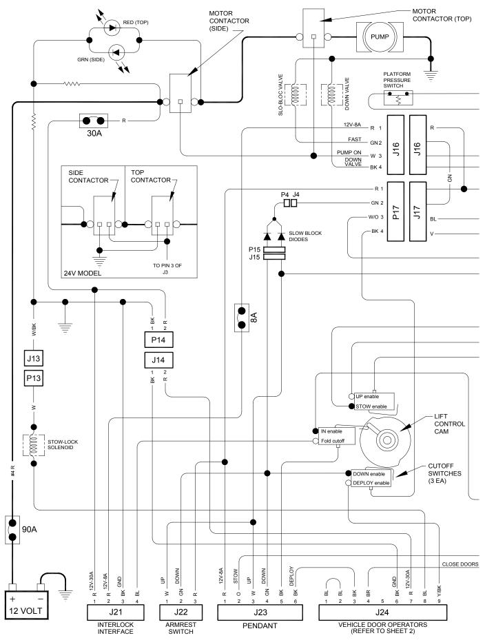
FIGURE 3-46: SLIDE-AWAY DOT PRIVATE USE LIFT SCHEMATIC - SHEET 1
