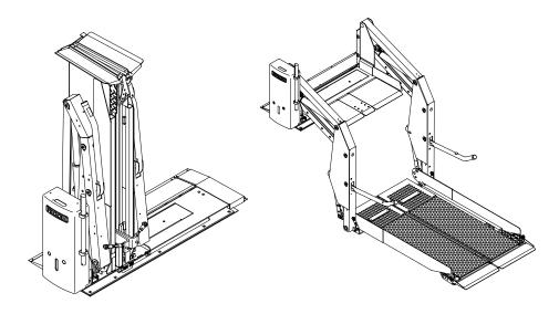
The lift control switches are used to unfold the platform from the vehicle (deploy). The exiting passenger then boards the large non-skid platform and the operator lowers the platform to the ground. After the passenger departs, the platform is raised and folded into the vehicle (stow). The platform folds vertically and the tower slides to the left after rising above floor level.
