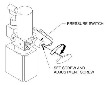
FIGURE 2-16: HYDRAULIC PUMP WITH PRESSURE SWITCH
