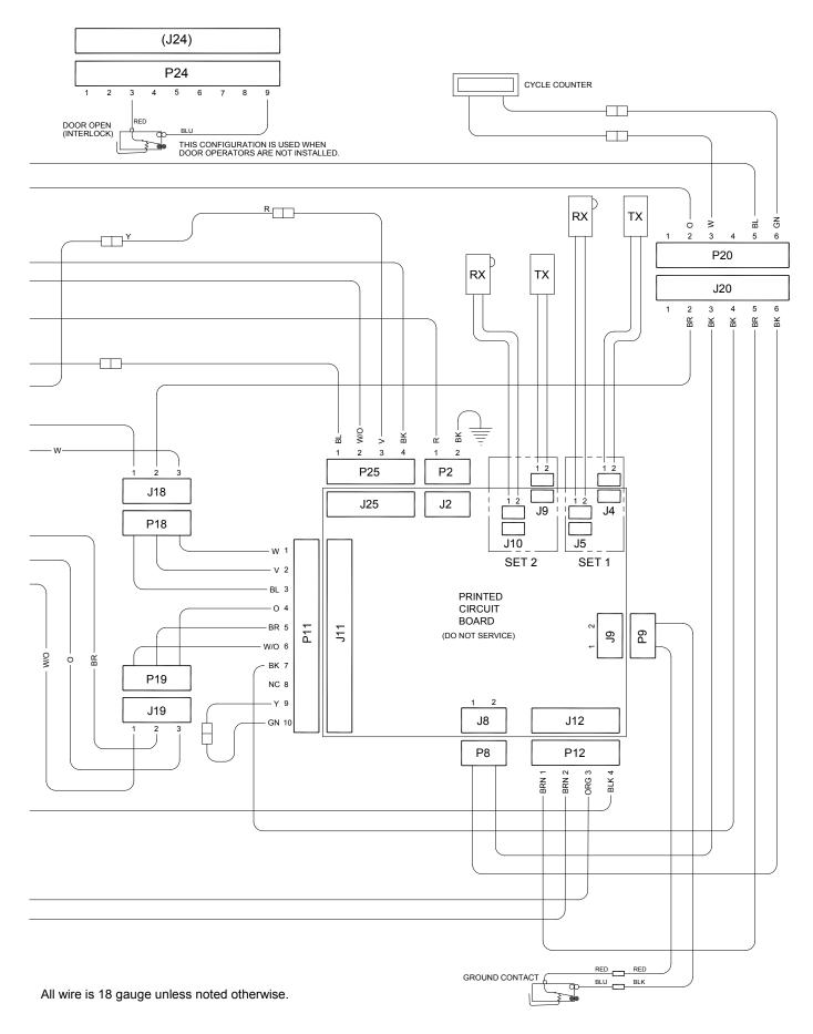
FIGURE 3-47: SLIDE-AWAY DOT PRIVATE USE LIFT SCHEMATIC - SHEET 2
