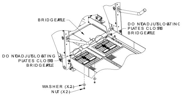
FIGURE 2-14: WHEELCHAIR LOCATING PLATE ADJUSTMENT
