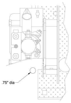
FIGURE 2-5: POWER CABLE ACCESS HOLE
