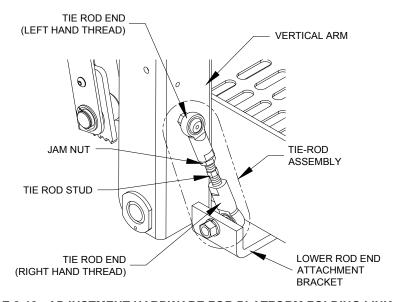
FIGURE 2-12: ADJUSTMENT HARDWARE FOR PLATFORM FOLDING LINKAGE
