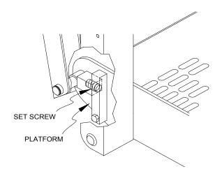
FIGURE 2-11: PLATFORM SET SCREWS
