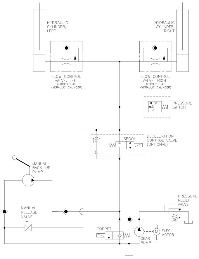
FIGURE 3-2: K-SERIES HYDRAULIC CIRCUIT DIAGRAM
