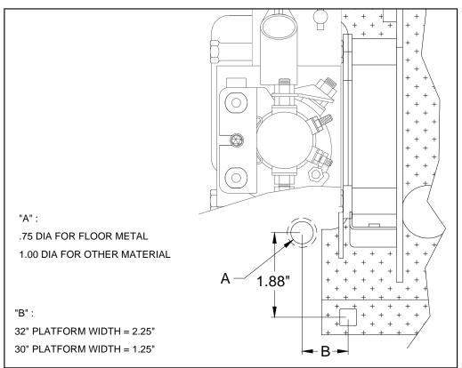
FIGURE 2-10: POWER CABLE ACCESS HOLE
