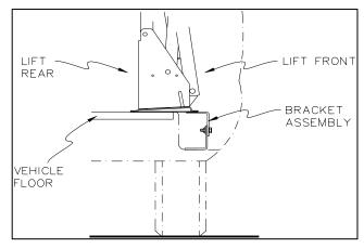
FIGURE 2-4: BRACKET ASSEMBLY
