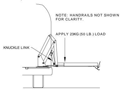
FIGURE 2-21: PRESSURE SWITCH TEST AT FLOOR LEVEL
