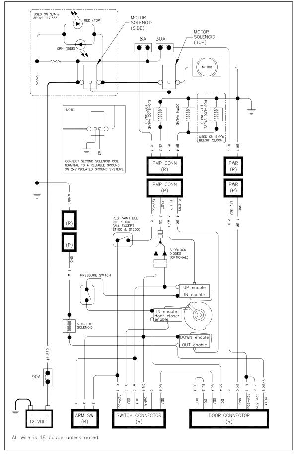
FIGURE 3-7: WIRING DIAGRAM FOR LIFT WITH DOOR OPERATOR
