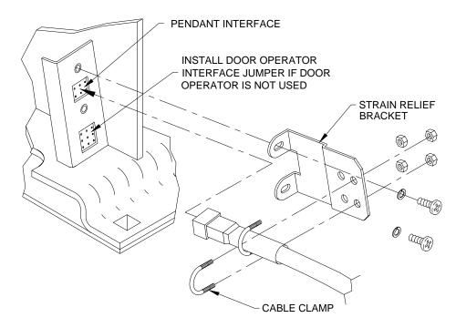
FIGURE 2-12: CONTROL INTERFACE AND STRAIN RELIEF
