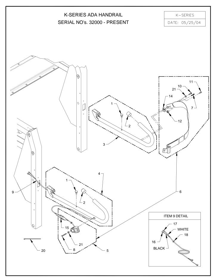
FIGURE 4-15: ADA HANDRAIL ASSEMBLIES
