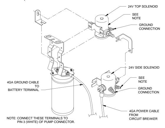
FIGURE 2-13: 24VDC WIRING
