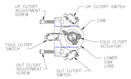
FIGURE 2-17: LIMIT SWITCH ADJUSTMENT DIAGRAM
