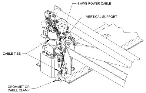
FIGURE 2-11: CABLE ROUTING
