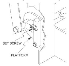
FIGURE 2-19: PLATFORM SET SCREWS
