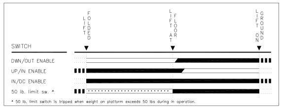
FIGURE 3-6: LIMIT SWITCH ACTUATION DIAGRAM
