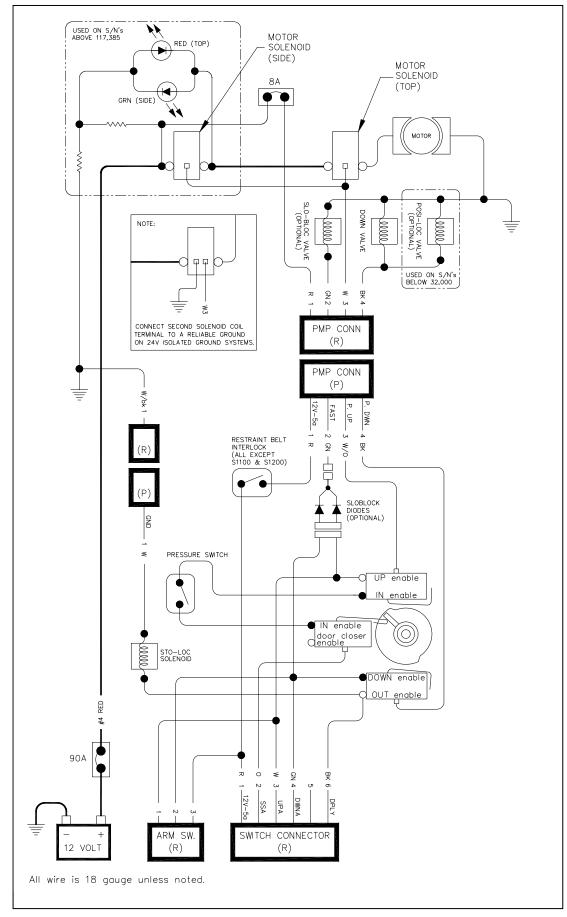
FIGURE 3-8: WIRING DIAGRAM FOR LIFT WITHOUT DOOR OPERATOR
