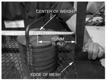
FIGURE 2-24: ALTERNATE 23KG (50 LB.) WEIGHT
