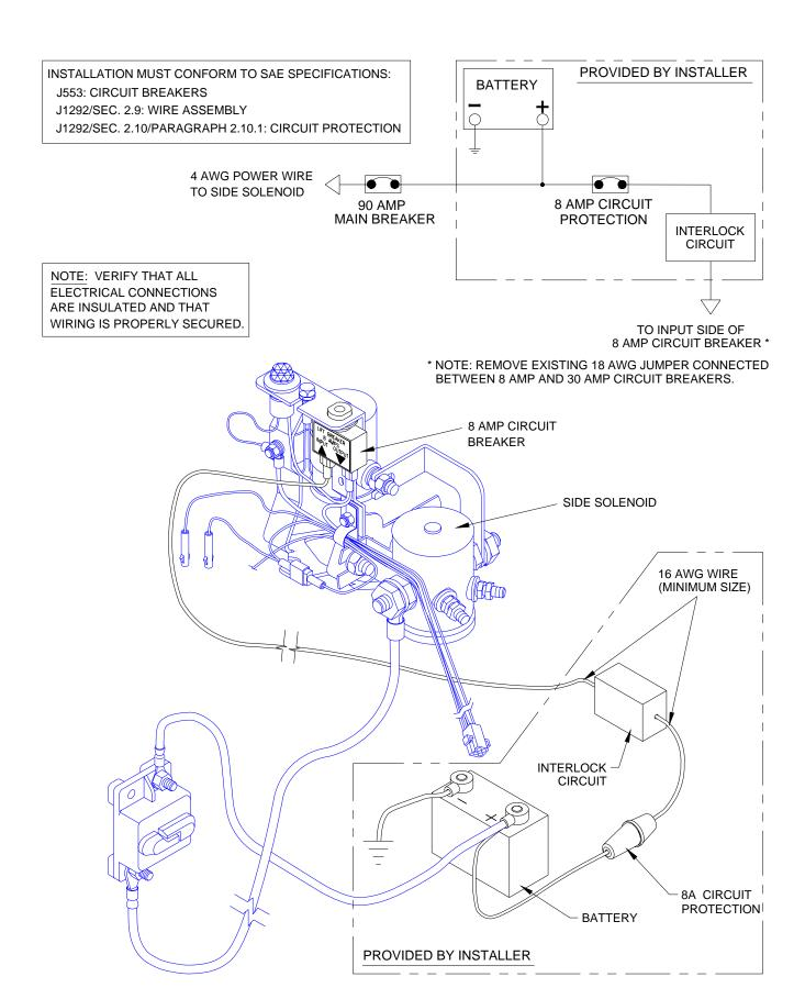
FIGURE 2-15: INTERLOCK METHOD #2
