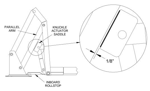
FIGURE 2-18: KNUCKLE ACTUATOR SADDLE MINIMUM CLEARANCE
