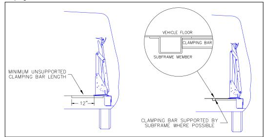
FIGURE 2-2: FORD VAN CLAMPING BAR ARRANGEMENT
