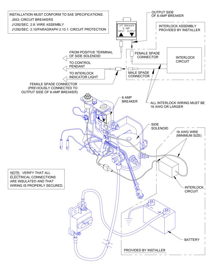
FIGURE 2-14: INTERLOCK METHOD #1
