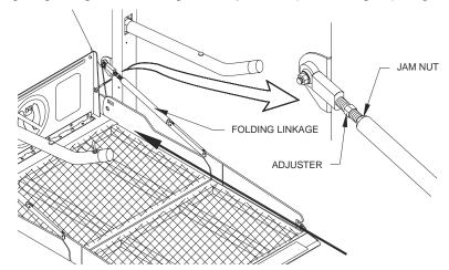
FIGURE 2-20: ADJUSTMENT HARDWARE FOR PLATFORM FOLDING LINKAGE
