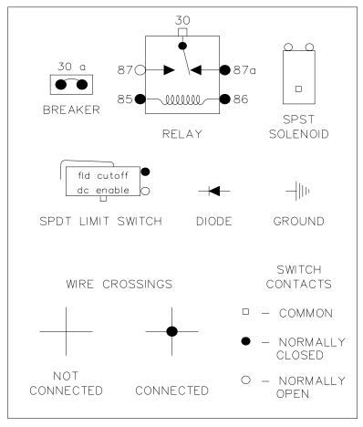
FIGURE 3-5: ELECTRICAL WIRING DIAGRAM SYMBOLS
