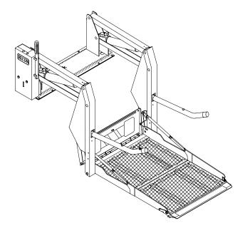
By using the lift control switches, the platform is unfolded from the vehicle (deployed). The passenger boards the large non-skid platform and the operator uses the control switches to gently lower the platform to the ground. After the passenger departs, the platform is raised and folded into the vehicle (stowed). The lift platform splits and folds horizontally when stowed.
