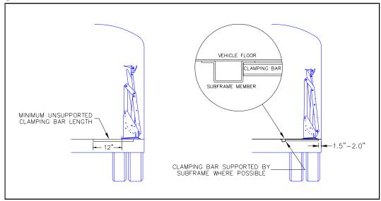
FIGURE 2-7: BUS CLAMPING BAR ARRANGEMENT
