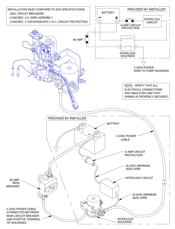
FIGURE 2-16: INTERLOCK METHOD #3
