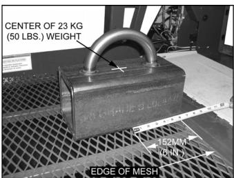
FIGURE 2-23: 23KG (50 LBS.) WEIGHT PLACEMENT ON PLATFORM
