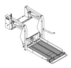
By using lift control switches, the lift is unfolded out from vehicle (deployed). The user boards the large non-skid platform and the operator uses control switches to gently lower platform to ground. After user departs, the platform is raised and folded into vehicle (stowed). The lift is also available with a platform that splits and folds when lift is stowed, providing easy vehicle access through the lift.
