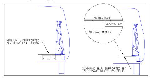
FIGURE 2-2: FORD VAN CLAMPING BAR ARRANGEMENT
