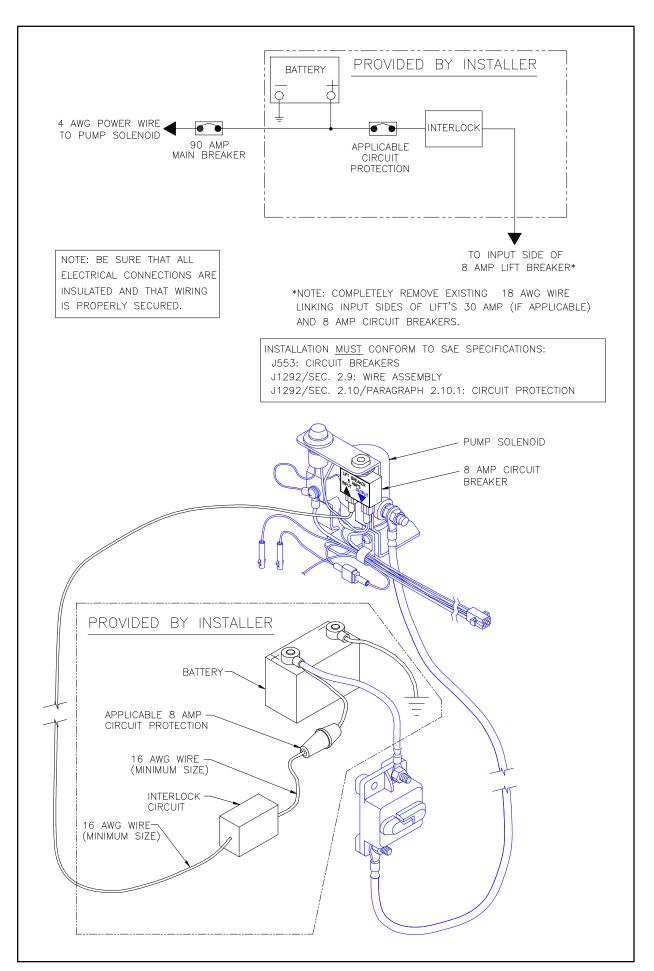
FIGURE 2-15: INTERLOCK METHOD #2
