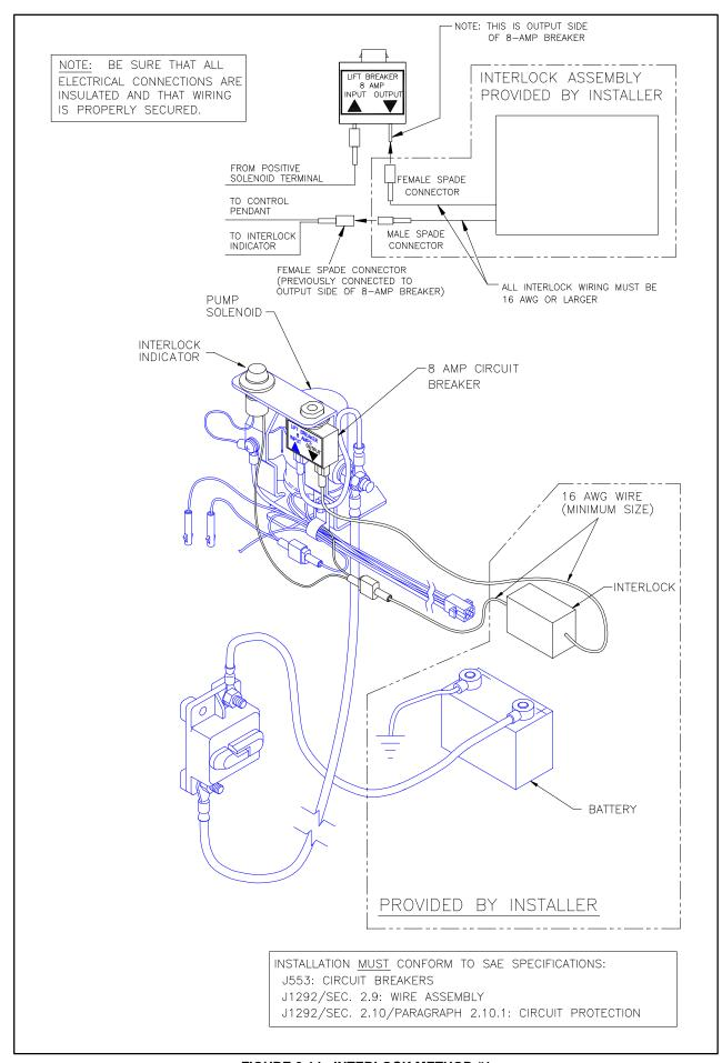
FIGURE 2-14: INTERLOCK METHOD #1
