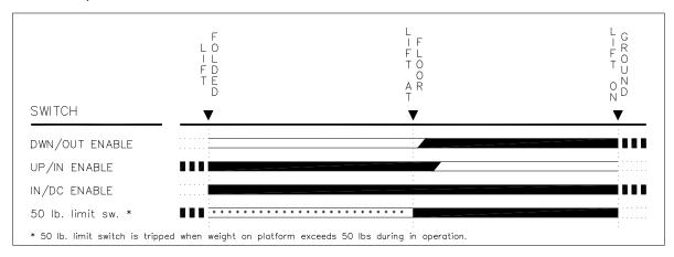
FIGURE 3-5: LIMIT SWITCH ACTUATION
