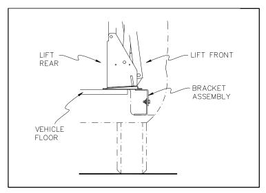
FIGURE 2-4: BRACKET ASSEMBLY
