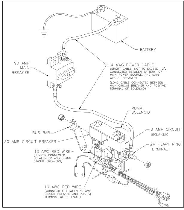
FIGURE 2-9: ELECTRICAL INSTALLATION DIAGRAM
