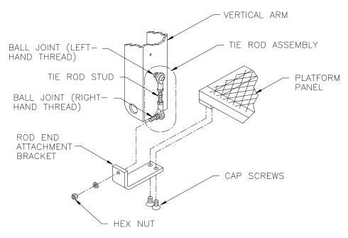
FIGURE 2-20: ROD END INSTALLATION
