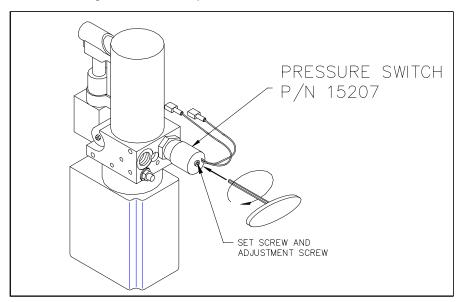
FIGURE 2-22: HYDRAULIC PUMP WITH PRESSURE SWITCH
