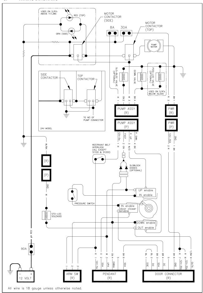
FIGURE 3-6: WIRING DIAGRAM FOR LIFT W/DOOR OPERATOR
