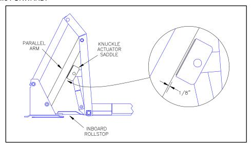
FIGURE 2-18: LIMIT SWITCH ADJUSTMENT CLEARANCE
