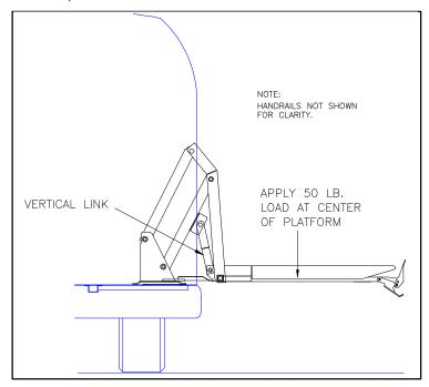
FIGURE 2-21: PRESSURE SWITCH TEST AT FLOOR LEVEL
