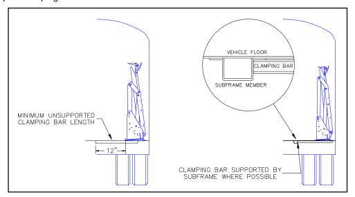
FIGURE 2-7: BUS CLAMPING BAR ARRANGEMENT
