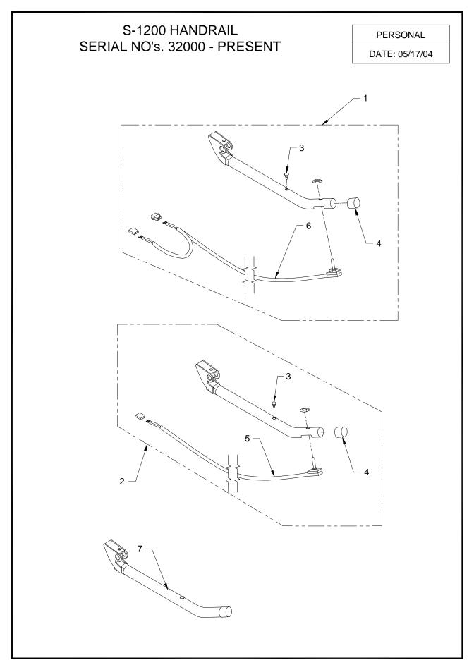
FIGURE 4-9: S-1200 HANDRAIL SERIAL NO'S. 32000 - PRESENT
