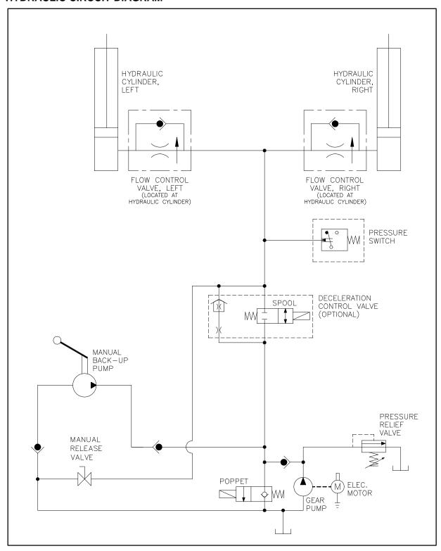
FIGURE 3-2: S-SERIES HYDRAULIC CIRCUIT
