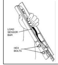
FIGURE 2-23: LOAD SENSOR ADJUSTMENT
