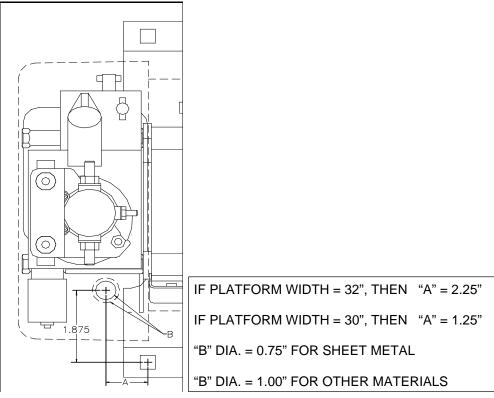
FIGURE 2-10: POWER CABLE ACCESS HOLE
