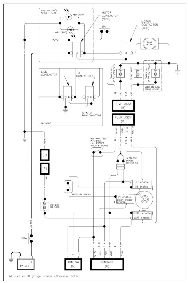
FIGURE 3-7: WIRING DIAGRAM FOR LIFT W/O DOOR OPERATOR 32DSSP02.C
