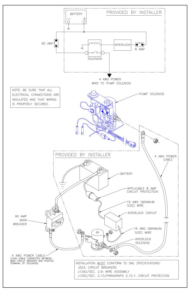
FIGURE 2-16: INTERLOCK METHOD #3
