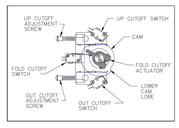
FIGURE 2-17: LIMIT SWITCH ADJUSTMENT DIAGRAM
