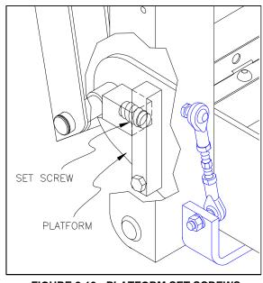
FIGURE 2-19: PLATFORM SET SCREWS
