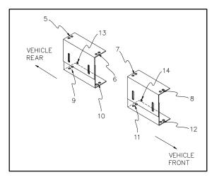
FIGURE 2-6: TOP BRACKET HOLE LOCATIONS
